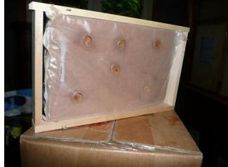
The evaporation frame contains wood shavings between two sheets of pierced plastic.
